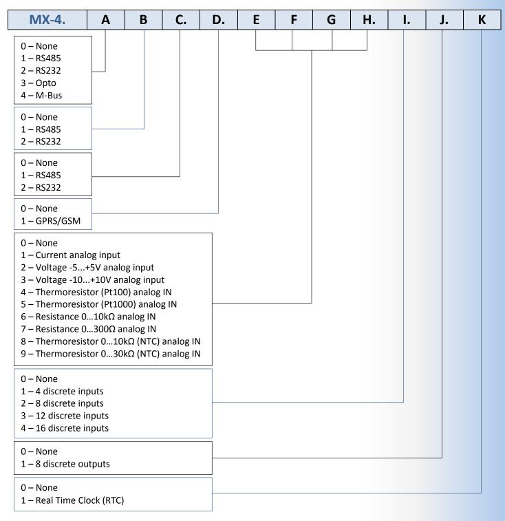
Example: MX-4.412.1.1400.2.8.1 (M-Bus, RS485, RS232, GPRS, Current Analog IN, Thermoresistor (Pt100) Analog IN, 8 Discrete IN, 8 Discrete OUT, RTC)
